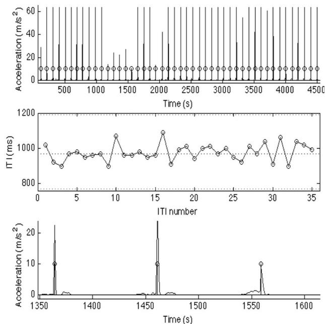
**Fig. 2** Graphical examples (from top to bottom) of (1) accelerometer movement data (minus the first ten excluded taps; circles denote local maxima), (2) series of corresponding inter-tap intervals, and (3) three individual taps from graph 1 (enlarged for clarity)
