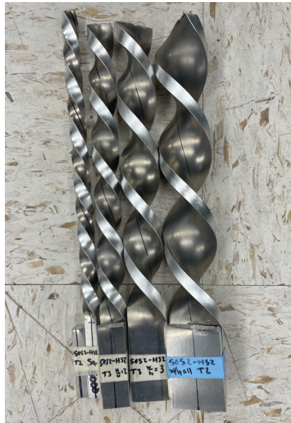
Figure 3.29 5052-H32 rupture specimens.
