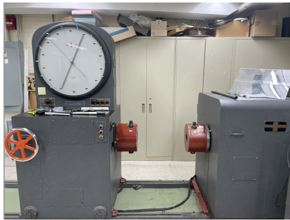
Figure 3.9 Torsion Machine that was used to run experiments.
