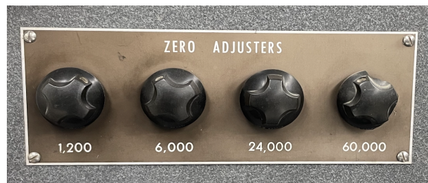
Figure 3.12 Knobs that zero the torsion machine.
