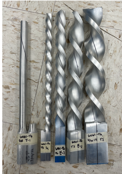
Figure 3.25 6061-T6 rupture specimens.
