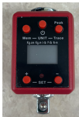
Figure 3.18 Frontal Image of Torque calibration device.
