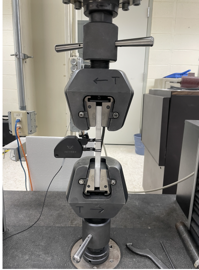
Figure 3.4 Tension specimen and extensometer arrangement.
