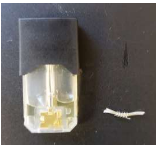
Figure 2. A JUUL pod that contains the e-liquid, heating element, and wick (left). A heating element and wick for better visual (right). This shows visually how the heating element and wick are directly in contact with the e-liquid.
