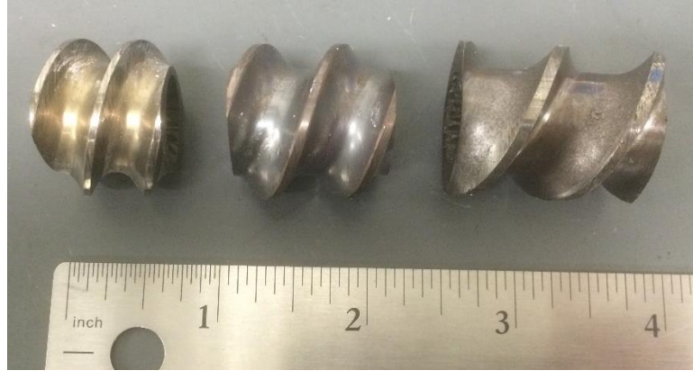
Figure 4.1.1: From left to right: small, medium, and large conveying elements used in Bucknell's SSSP machine
