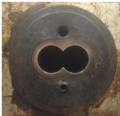
Figure 2.2.5: Cross section of the ZE-25 extruder barrels
