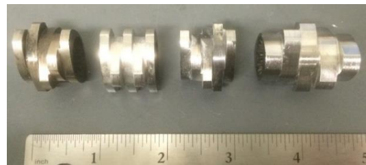
Figure 2.2.4: Kneading elements used in Bucknell's SSSP machine; from left to right, small forward, small neutral, small reverse, large forward
