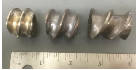
Figure 2.2.3: From left to right; small, medium, and large conveying elements used in Bucknell's SSSP machine
