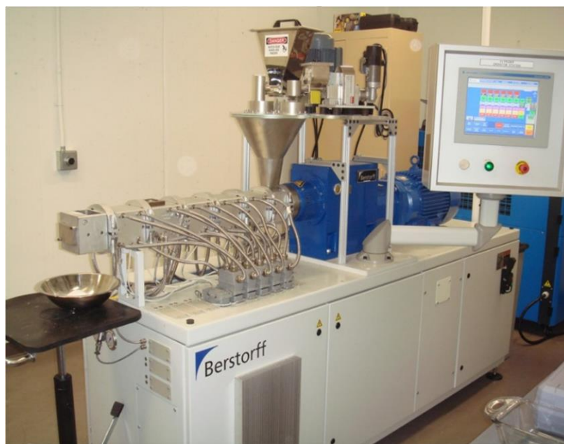
Figure 2.2.1: The KraussMaffei Berstorff ZE-25 UTX extruder at Bucknell University
