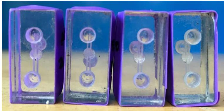
*Fig. 18. Pneumatic AND gates fabricated using laser engraving and adhesive method with varying channel depths of 2.7 mm, 1.5 mm, 0.8 mm, and 0.5 mm (from left to right).*
