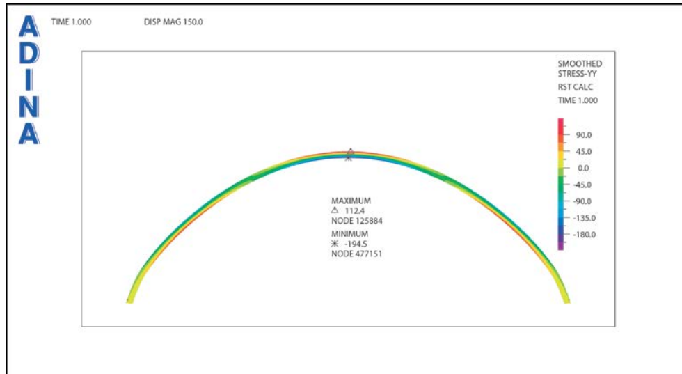
Figure 38. Radial stresses (psi) at the mid-span cross-section of FEM-4
