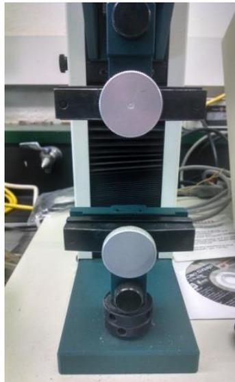
**Figure 17:** Tensile tester with soft grip attachment
