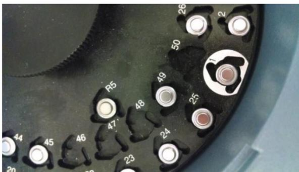
**Figure 13:** Clamped hermetic pans within the DSC. Pan R5 is a reference pan and all others contain samples to be tested.
