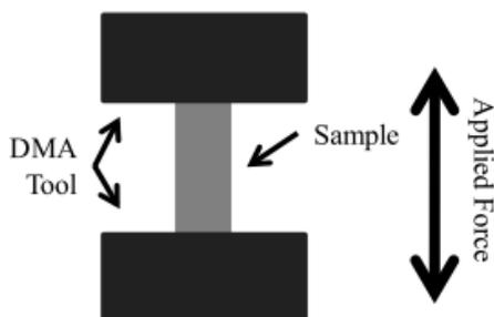
**Figure 14:** Diagram of DMA testing apparatus showing the direction of tension on a sample
