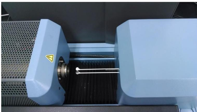
**Figure 15:** Opened TGA showing the balance and alumina pan
