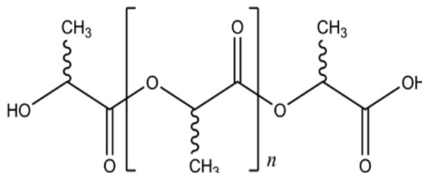
**Figure 1:** Chemical structure of PLA
