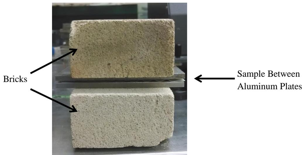
**Figure 12:** PLA sample cooling between two bricks
