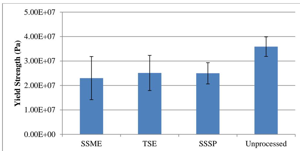
**Figure 26:** Average yield strength of each processing method. The error bars correspond to one standard deviation in our measurement
