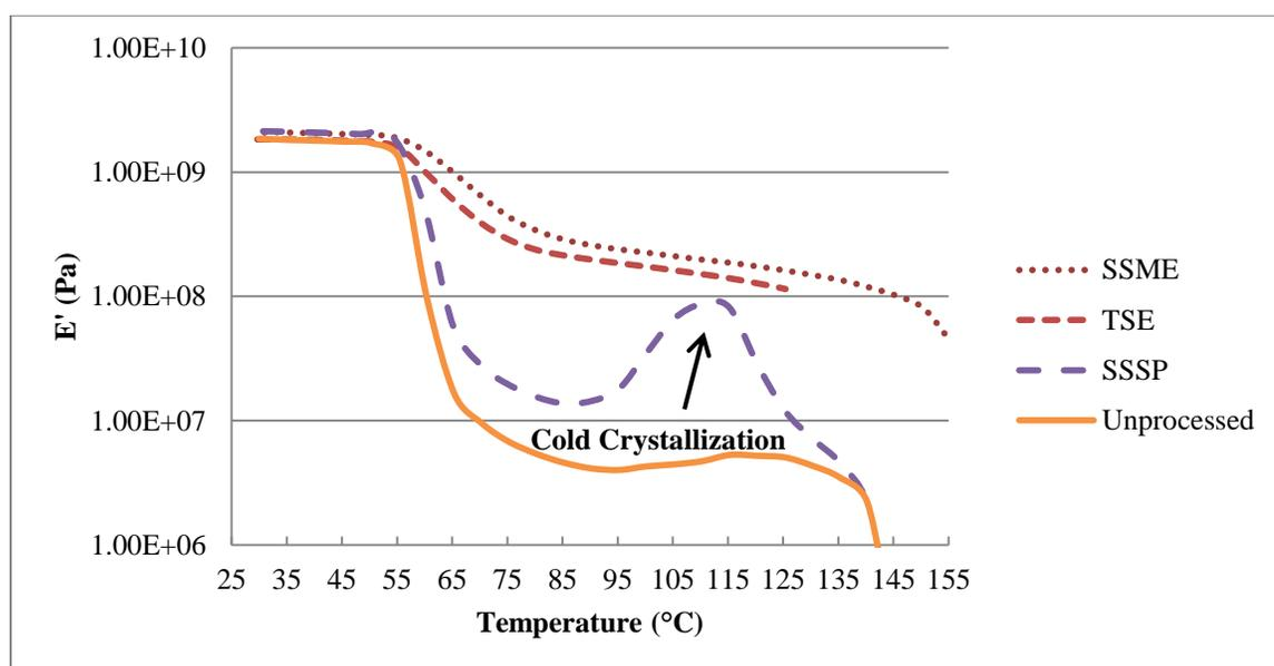
**Figure 21:** Storage modulus for each processed an unprocessed sample from 30°C to 155°C
