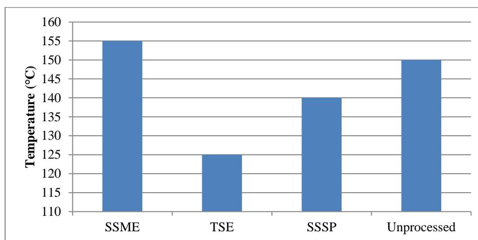
**Figure 23:** Softening temperature of each processing method
