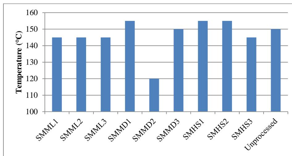
**Figure 32:** Softening temperature of SSME-processed PLA
