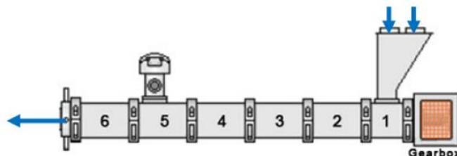
**Figure 10:** Diagram of KrausMaffei Berstorff ZE-25A UTX extruder showing Zones 2-6 can be temperature-controlled
