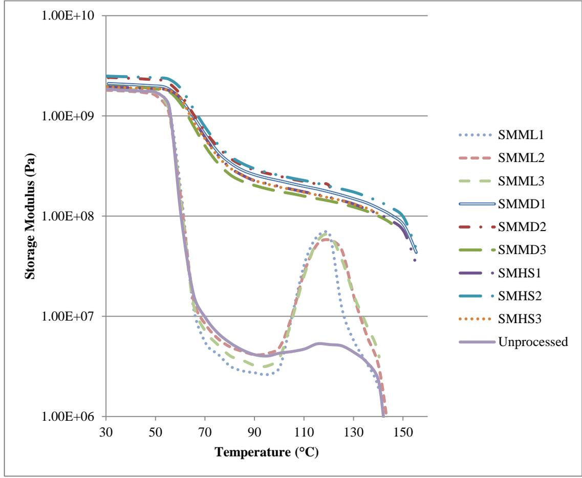
**Figure 31:** Storage modulus of SSME-processed PLA between 30-160°C
