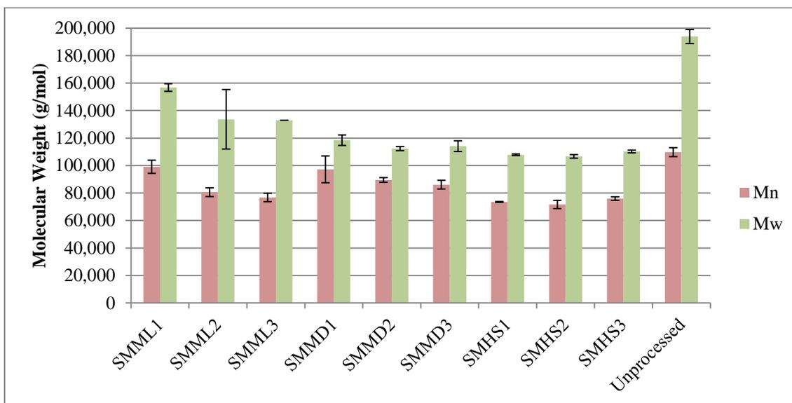
**Figure 34:**  $M_n$  and  $M_w$  for all SSME-processed PLA samples. All error bars represent one standard deviation between the two reported trials
