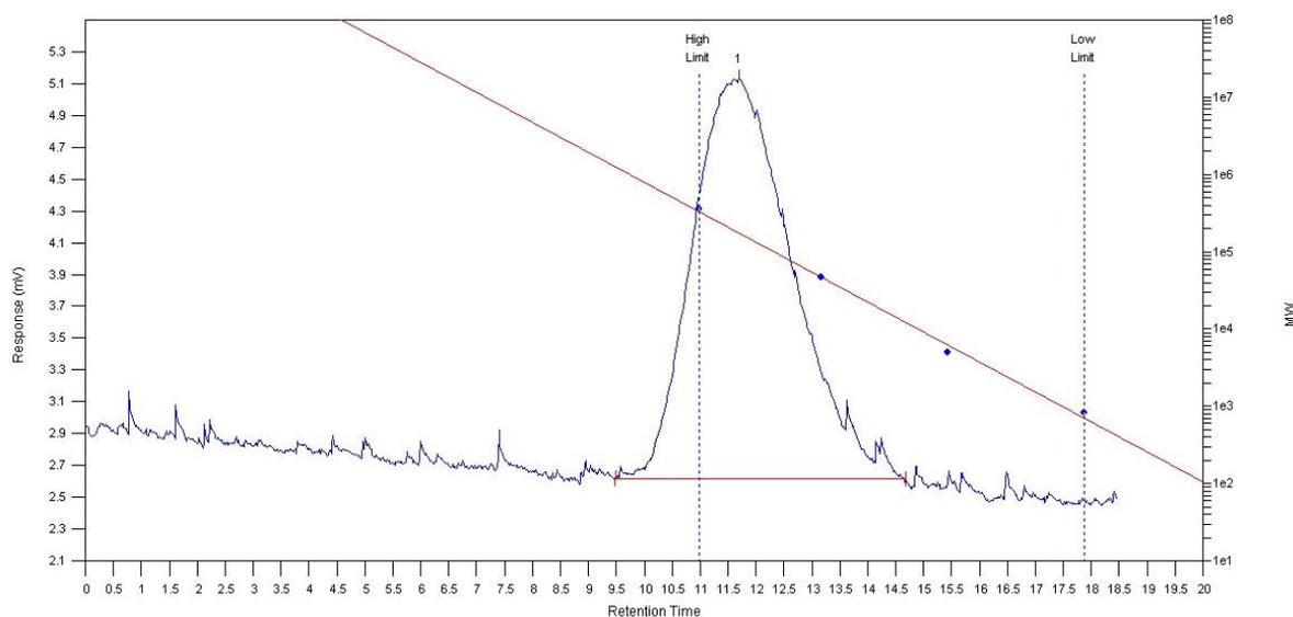
**Figure 16:** Sample GPC plot of response as a function of retention time
