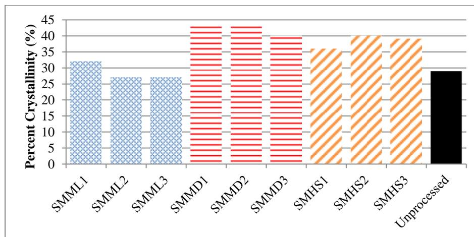
**Figure 29:** Percent crystallinity for all 9 SSME-processed PLA samples, measured via isothermal crystallization at 105°C
