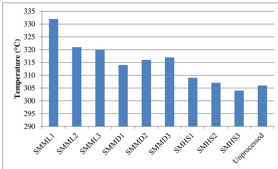
**Figure 33:** Degradation temperature for each SSME-processed sample, defined as the temperature at a 5% mass loss
