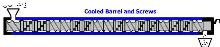
**Figure 4:** Diagram depicting SSSP processing
