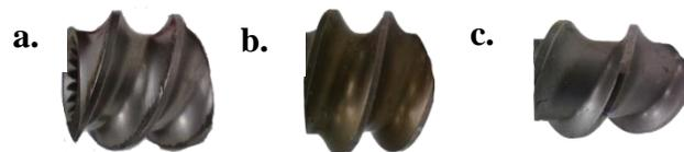
**Figure 8:** **a.** Short conveying element **b.** Medium conveying element
