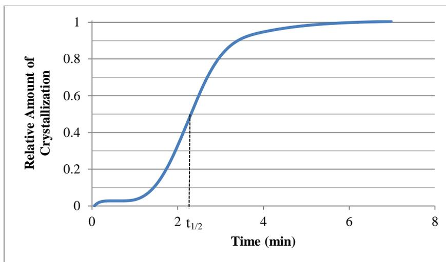
**Figure 19:** Example crystallization curve showing crystallization half time ( $t_{1/2}$ )
