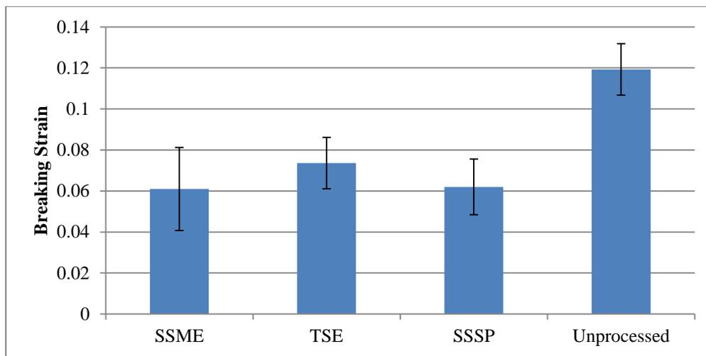
**Figure 27:** Average breaking strain of PLA processed through each method. The error bars correspond to one standard deviation in our measurement
