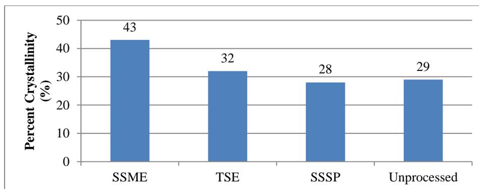
**Figure 18:** Percent crystallinity for each processing method
