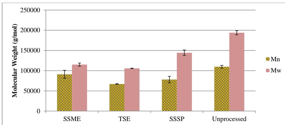
**Figure 25:**  $M_n$  and  $M_w$  for each processing technique. All error bars represent 1 standard deviation between the two reported trials
