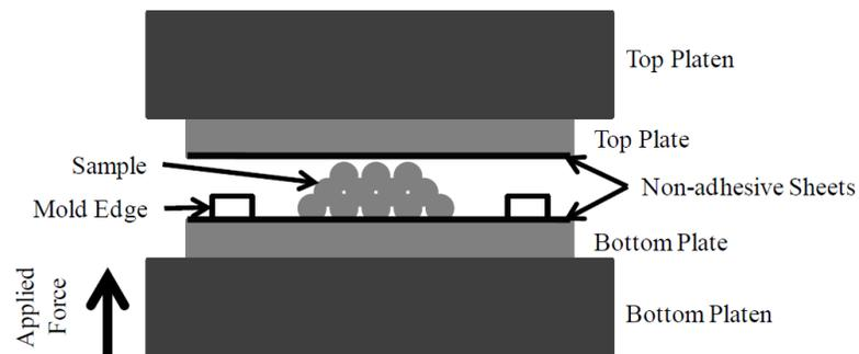
**Figure 11:** Schematic of sheet pressing procedure
