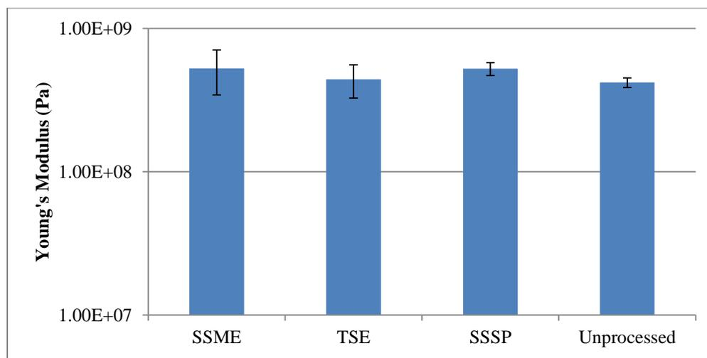
**Figure 28:** Average Young's modulus of PLA processed through each method. The error bars correspond to one standard deviation in our measurement
