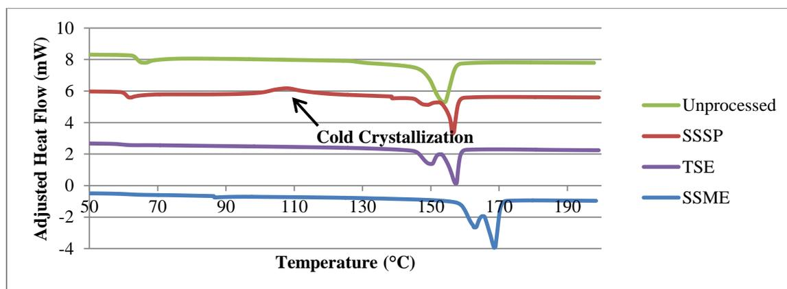
**Figure 20:** Non-isothermal DSC thermogram for each sample at a heating rate of  $5^{\circ}\text{C}/\text{min}$ . The curves were shifted in 3 mW increments for clarity
