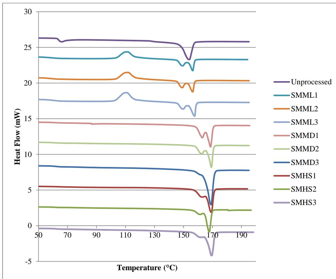
**Figure 30:** Heat flow for all SSME-processed PLA samples. All trials were shifted in 3 mW increments for clarity
