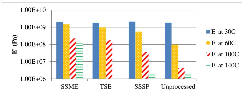
**Figure 22:** Storage moduli of PLA processed samples at 30°C, 60°C, 100°C, and 140°C
