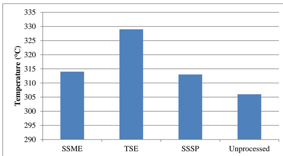
**Figure 24:** Degradation temperature for each processing technique at a 5% loss
