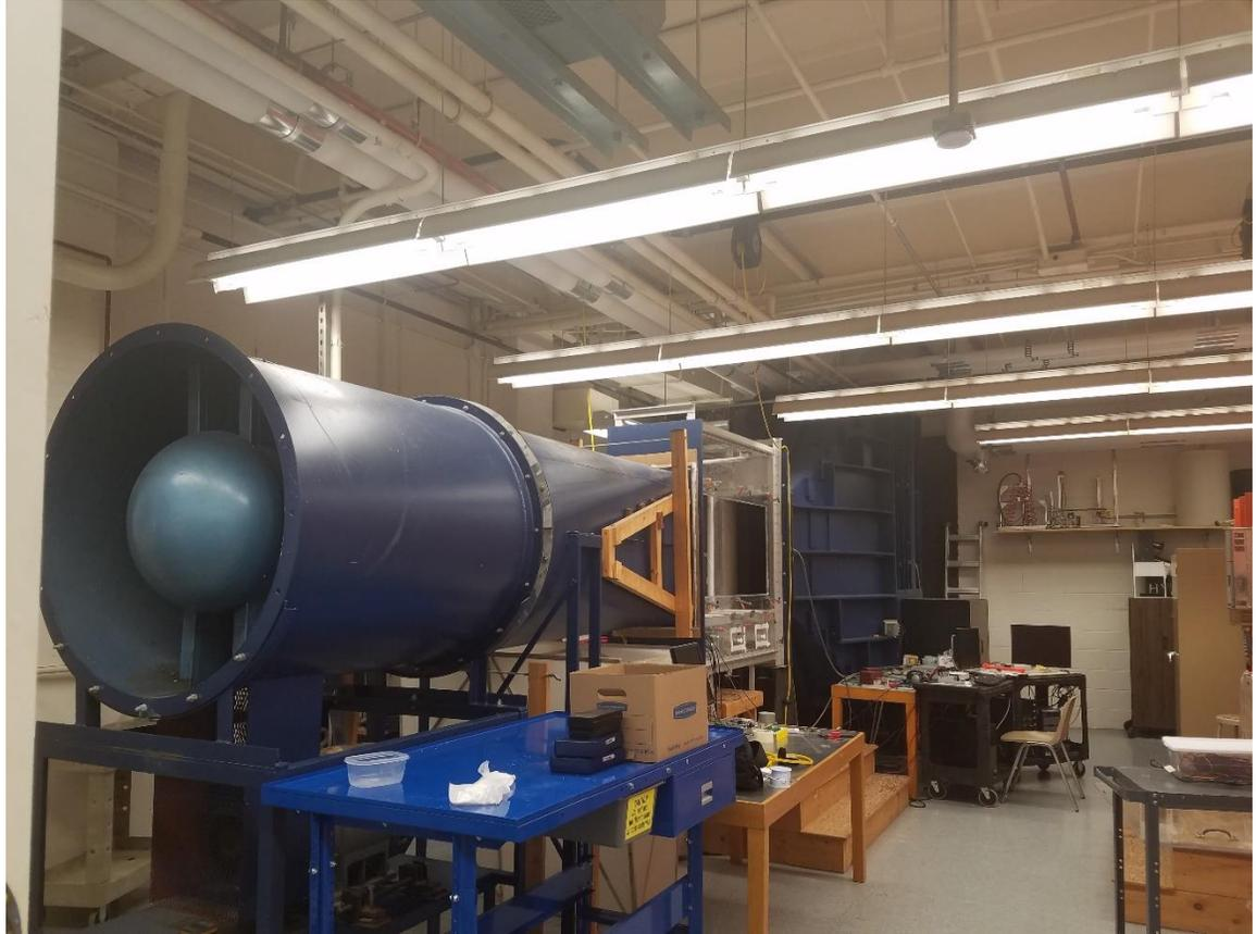
Figure 8 The subsonic open loop wind tunnel in the Mechanical Engineering Laboratory at Bucknell University
