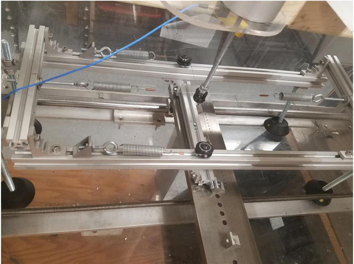
Figure 14 Mounted system with base, threaded rod, cylinder and springs
