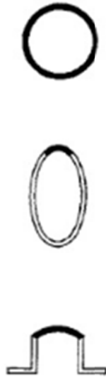
Figure 5. Sample of aluminum curved shapes as they appear within structural shapes (Kissell, 1995)
