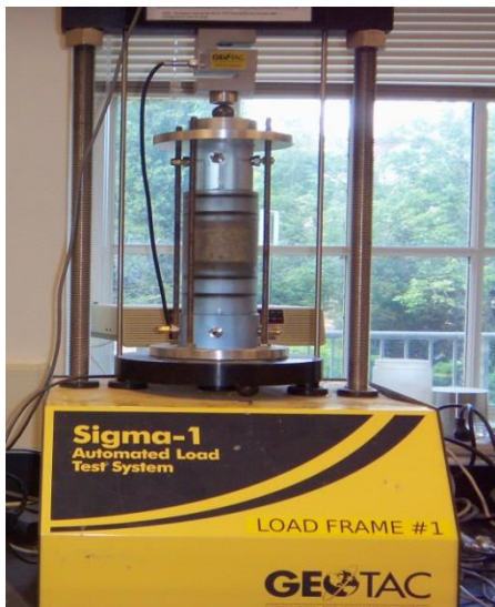
Figure 3.15 Load Frame-Sigma1 apparatus that was used to consolidate the bentonite slurry
