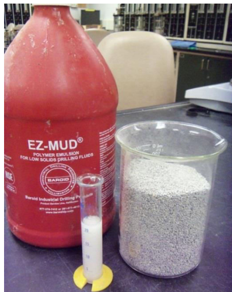
Figure 3.1 The constituents of the bentonite grout: BENSEAL® granules and EZ-MUD®
