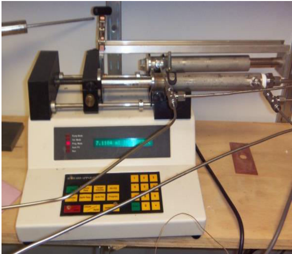
Figure 3.12 A PH 22/2000 Programmable Harvard Apparatus flow pump that was used for the hydraulic conductivity tests
