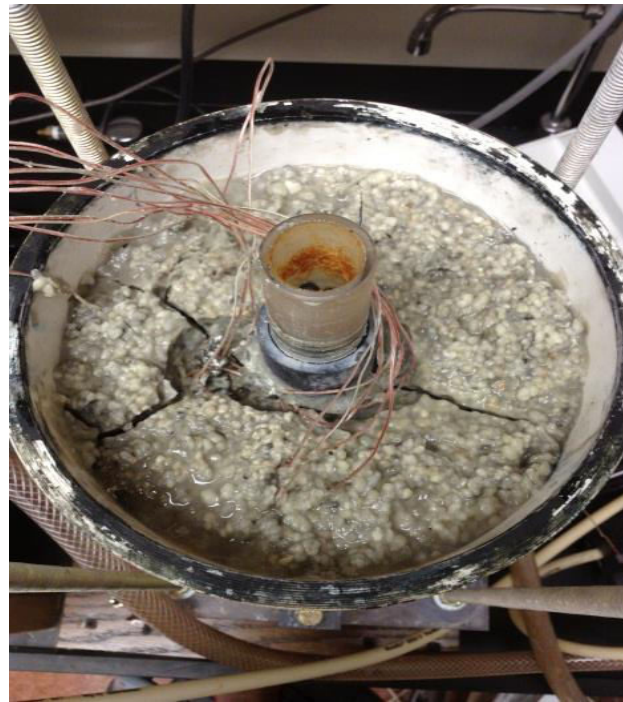
Figure 4.4 Picture of the geothermal well model with cracked bentonite grout after the thermal conductivity test were terminated.
