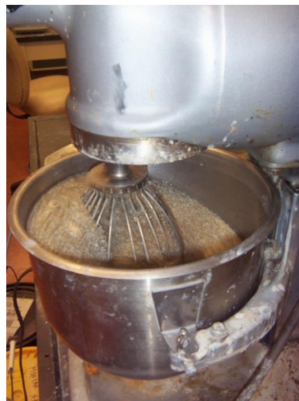
Figure 3.2 The BENSEAL/EZ-MUD® slurry being mixed in the Hobart mixer
