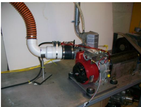
Figure 3-2: Briggs and Stratton 10 HP Configured to the Test Bench
