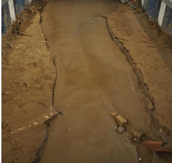
Figure 25 – Photograph of the resulting channel from trial 2 (facing upstream).
