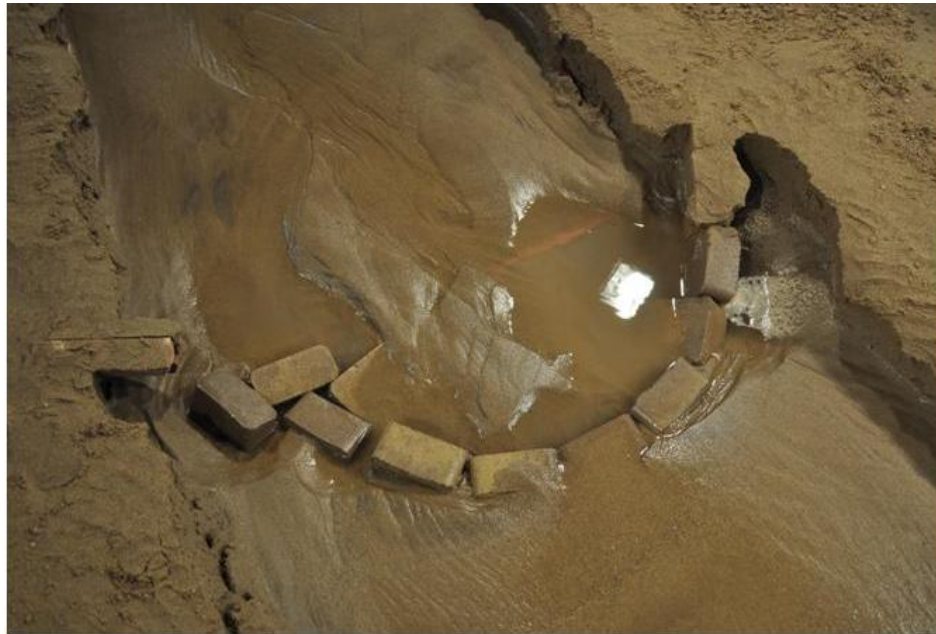
Figure 36 – Photograph of the downstream cross vane after trial 6.
