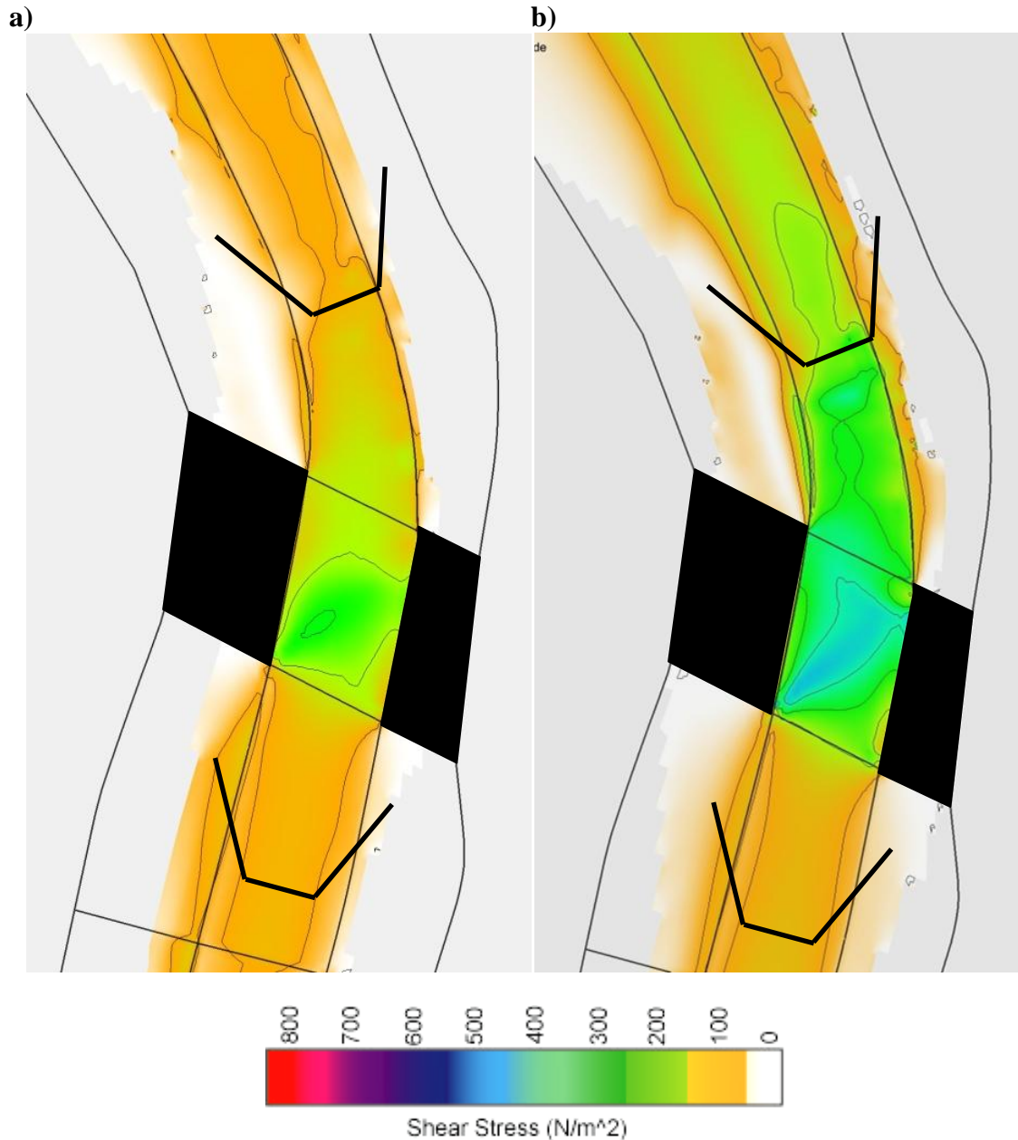
Figure 42 – FESWMS shear stress contours for the March 2012 survey at the two and ten year flow rates (a and b, respectively) (The black rectangles indicate the bridge (a 14 m x 21 m span) and approximate location of the restoration structures).
