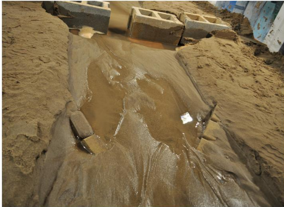
Figure 32 – Photograph of the upstream cross vane after trial 5 (facing downstream).
