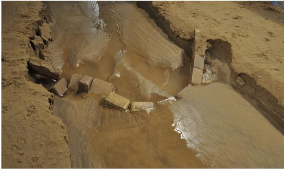
Figure 33 – Photograph of the downstream cross vane after trial 5 (facing downstream).
