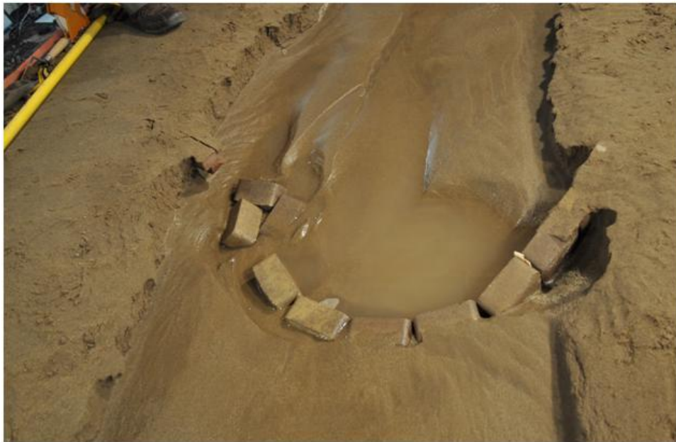
Figure 31 – Photograph of the downstream cross vane after trial 4 (facing downstream).
