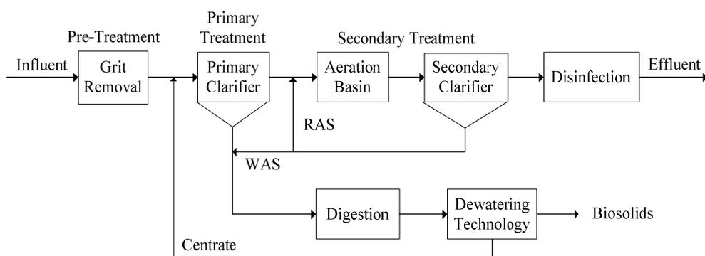
**Figure 1–1: Schematic for Wastewater Treatment Plant**
