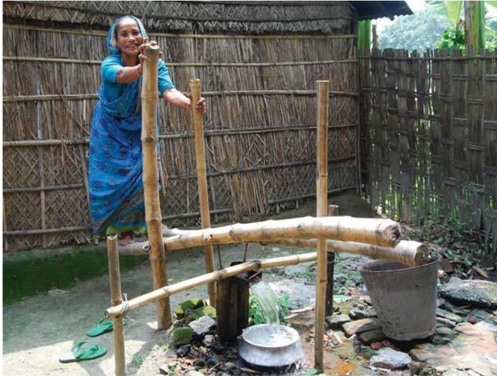
**Figure 4-2 IDE Treadle Pump [3]**
