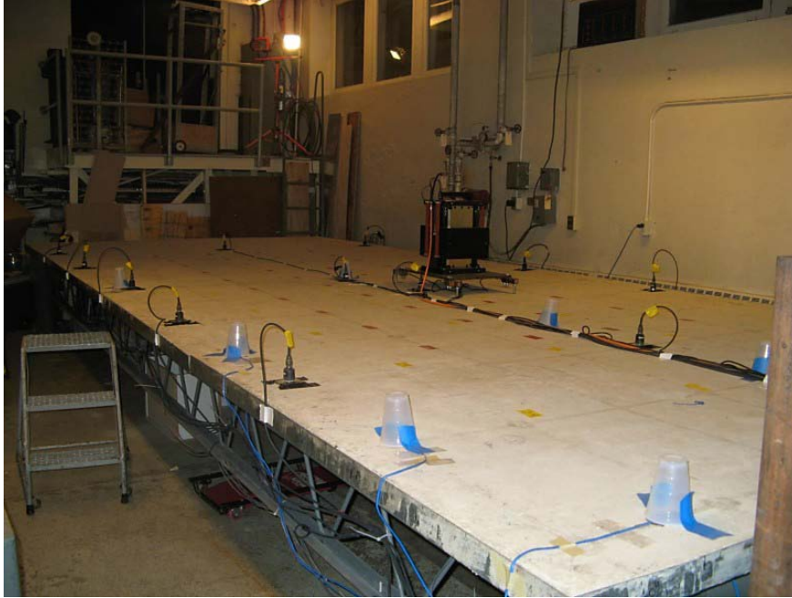
Figure 5: Empty structure with electrodynamic shaker and accelerometers shown.
