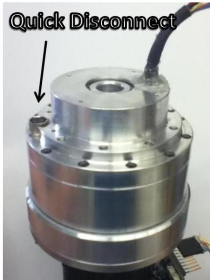
**Figure 58: Final Assembled Shoulder Joint**
