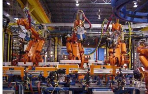
**Figure 3: GM spot weld assembly line [8]**
