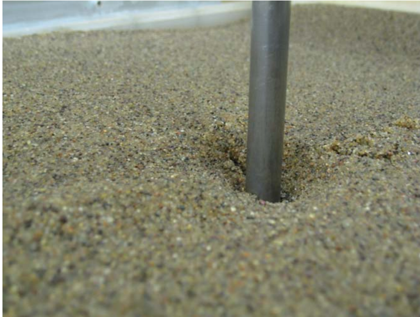
Figure 33: Erosion around cylinder in test section.
