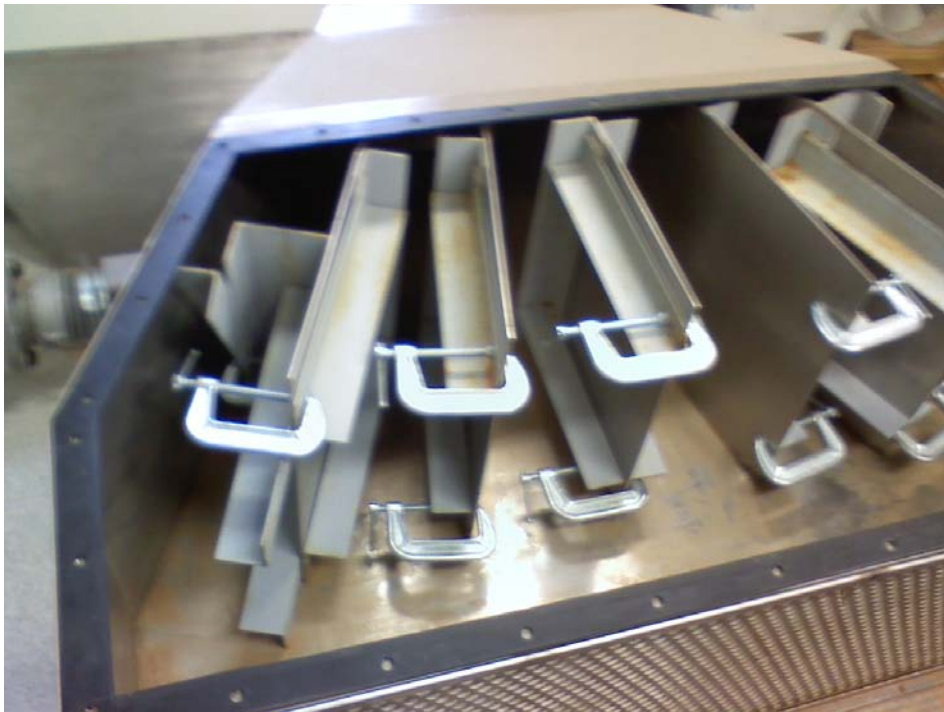
Figure 19: Flow conditioning devices in diffuser.
