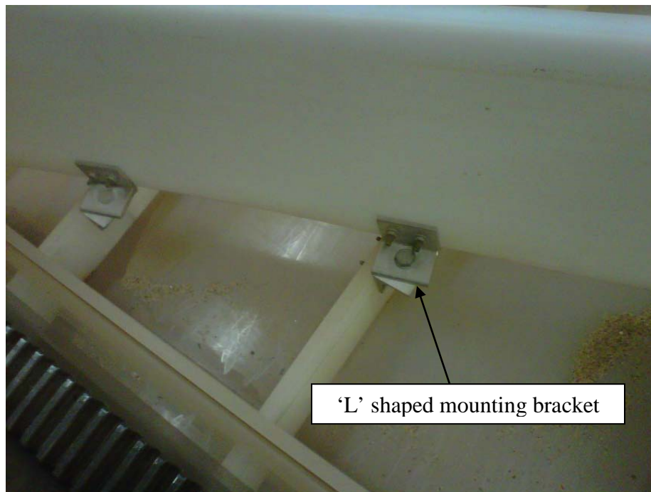
Figure 28: Mounting brackets for diffusing section of nozzle.
