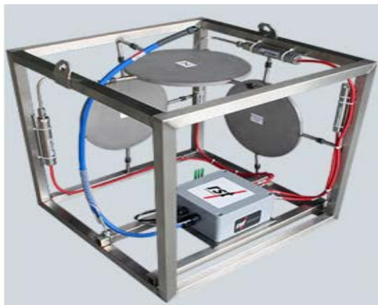
Figure 9. Photograph of earth pressure cell cage (RST Instruments, Maple Ridge, BC, Canada).
