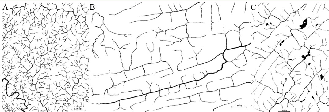
Figure 5 a) Dendritic drainage, northwestern part subsequent streams. of Palmyra (Va.) quadrangle. Scale 1:125,000. b) Trellis drainage, southern part of Williamsport (Pa.) quadrangle. Scale I: 62,500. c) Rectangular drainage, southwestern part of Elizabethtown (N.Y.) quadrangle. Scale 1:62,-500. (Images from: Zernitz 1932)
