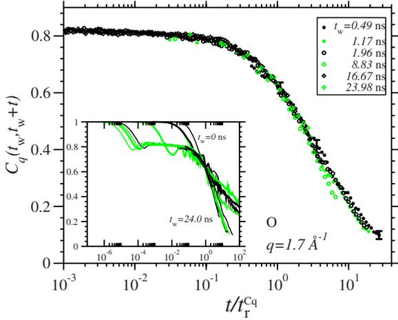
FIG. 8. (Color online)  $C_q(t_w, t_w+t)$  for the quench from  $T_i=2500$  K to  $T_f=5000$  K for O-atoms and  $q=1.7 \text{ \AA}^{-1}$ . Waiting times and corresponding lines in the inset are the same as in Fig. 4.
