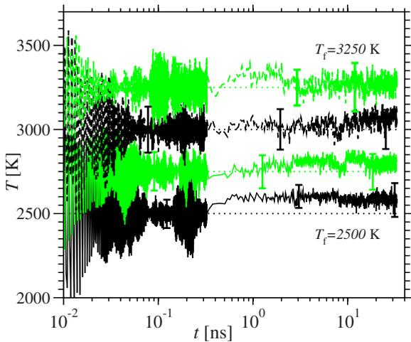
FIG. 2. (Color online) Temperature  $T = \frac{2\bar{E}_{\text{kin}}}{3N}$  as a function of time  $t$  for  $T_i=5000$  K,  $T_f=2500$ , 2750, 3000, and 3250 K shown in each case for the 11th independent simulation run.  $\bar{E}_{\text{kin}}$  includes a time average and error bars indicate the corresponding fluctuations.
